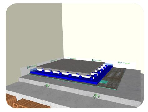
Cast of traditional concrete screed, possibly reinforced, with a thickness of about 50 mm above the insulation board bumps. The thickness of this layer will influence the choice of the most appropriate acoustic coating and determine the operation of the underfloor heating.
