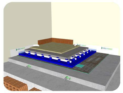
Install by gluing or floating system the finishing floor of any type and thickness. Only after this operation can the excess of the **POLYBAND AD** desolarizing strip be removed and the baseboard installed. It is recommended not to lay the baseboard completely on the floor but to leave a minimum of air blade and seal with elastic glue.
