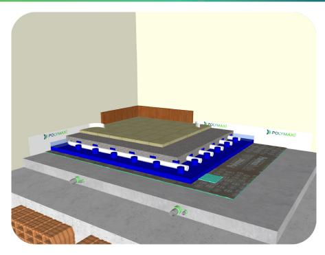
Install by gluing or floating system the finishing floor of any type and thickness. Only after this operation can the excess of the **POLYBAND AD** desolarizing strip be removed and the baseboard installed. It is recommended not to lay the baseboard completely on the floor but to leave a minimum of air blade and seal with elastic glue.
