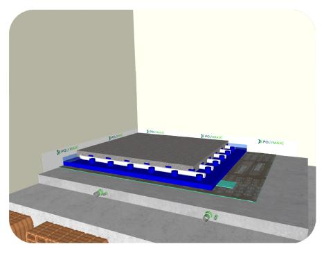
Cast of traditional concrete screed, possibly reinforced, with a thickness of about 50 mm above the insulation board bumps. The thickness of this layer will influence the choice of the most appropriate acoustic coating and determine the operation of the underfloor heating.
