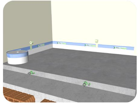
Apply the adhesive part of the **POLYBAND AD** desolarizing tape, removing the protective foil, at the base of the wall and support with some pieces of tape the protective nylon that must be laid on top of the radiant panel. The strip is laid with the shorter side of the nylon-strip fastening towards the lightened screed. This application must be carried out continuously on the entire perimeter of the rooms to be treated.
