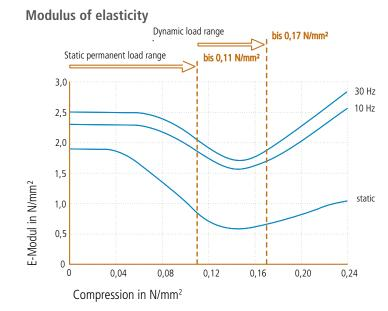
Load dependence of the static and dynamic moduli of elasticity. Dynamic E-modulus: harmonic excitation with an amplitude of  $\pm$  0.22 mm at 10 Hz and  $\pm$  0.08 mm at 30 Hz. Static E-modulus: tangent modulus from the spring characteristic. Measurement according to DIN 53513. Form factor q = 3.
