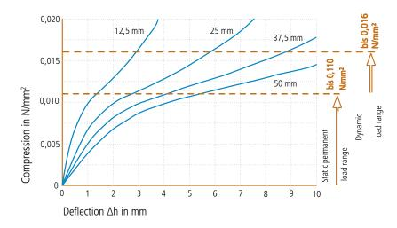
Spring characteristic curve. Test speed  $v=1\,\%$  of thickness. Test at room temperature between flat steel plates. Recording of the 3rd load. Form factor q=3.
