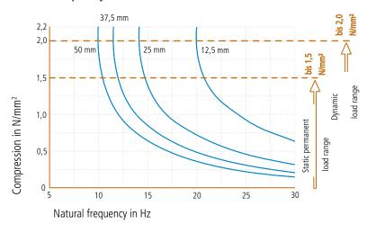
Natural frequency of a system consisting of a rigid mass and a layer of ISOLMER® on a rigid base. Form factor q=2.
