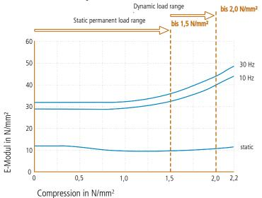
Load dependence of the static and dynamic moduli of elasticity. Dynamic E-modulus: harmonic excitation with an amplitude of  $\pm$  0.22 mm at 10 Hz and  $\pm$  0.08 mm at 30 Hz. Static E-modulus: tangent modulus from the spring characteristic.
