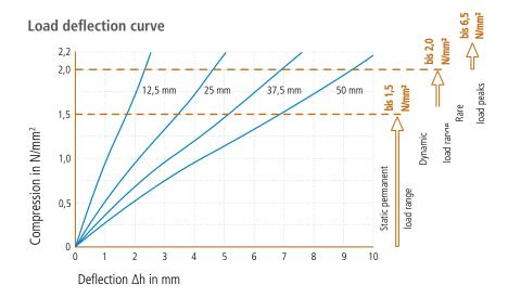
Spring characteristic curve. Test speed  $v=1\,\%$  of thickness. Test at room temperature between flat steel plates. Recording of the 3rd load. Form factor q=2.
