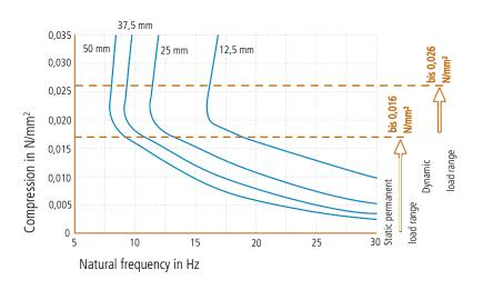
Natural frequency of a system consisting of a rigid mass and a layer of ISOLMER® on a rigid base. Form factor q=3.
