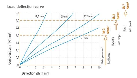
Spring characteristic curve. Test speed  $v=1\,\%$  of thickness. Test at room temperature between flat steel plates. Recording of the 3rd load. Form factor q=1.25.
