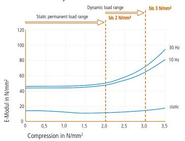
Load dependence of the static and dynamic moduli of elasticity. Dynamic E-modulus: harmonic excitation with an amplitude of  $\pm$  0.22 mm at 10 Hz and  $\pm$  0.08 mm at 30 Hz. Static E-modulus: tangent modulus from the spring characteristic. Measurement according to DIN 53513.
