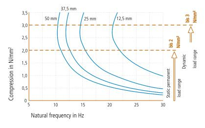
Natural frequency of a system consisting of a rigid mass and a layer of ISOLMER® on a rigid base. Form factor q=1.25.
