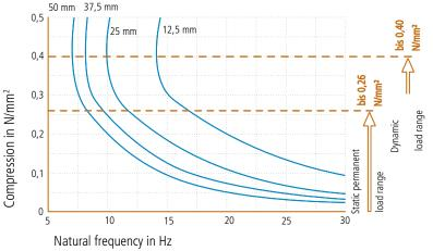
Natural frequency of a system consisting of a rigid mass and a layer of ISOLMER<sup>®</sup> on a rigid base. Form factor q = 3.
