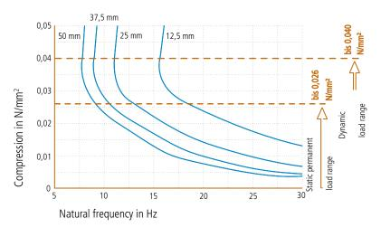
Natural frequency of a system consisting of a rigid mass and a layer of ISOLMER® on a rigid base. Form factor q=3.
