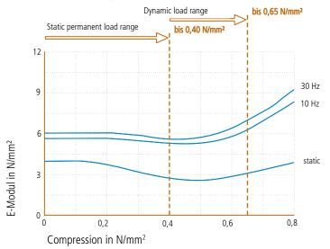
Load dependence of the static and dynamic moduli of elasticity. Dynamic E-modulus: harmonic excitation with an amplitude of  $\pm$  0.22 mm at 10 Hz and  $\pm$  0.08 mm at 30 Hz. Static E-modulus: tangent modulus from the spring characteristic. Measurement according to DIN 53513. Form factor q = 3.
