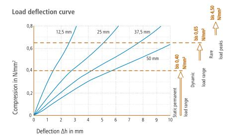
Spring characteristic curve. Test speed  $v=1\,\%$  of thickness. Test at room temperature between flat steel plates. Recording of the 3rd load. Form factor q=3.
