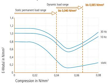
Load dependence of the static and dynamic moduli of elasticity. Dynamic E-modulus: harmonic excitation with an amplitude of  $\pm$  0.22 mm at 10 Hz and  $\pm$  0.08 mm at 30 Hz. Static E-modulus: tangent modulus from the spring characteristic. Measurement according to DIN 53513. Form factor q = 3.
