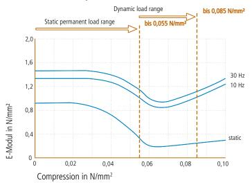
Load dependence of the static and dynamic moduli of elasticity. Dynamic E-modulus: harmonic excitation with
