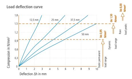
Spring characteristic curve. Test speed v = 1 % of thickness. Test at room temperature between flat steel Recording of the 3rd load. Form factor q = 2.
