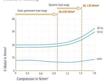
Load dependence of the static and dynamic moduli of elasticity. Dynamic E-modulus: harmonic excitation with an amplitude of  $\pm$  0.22 mm at 10 Hz and  $\pm$  0.08 mm at 30 Hz. Static E-modulus: tangent modulus from the
