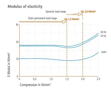
Load dependence of the static and dynamic moduli of elasticity. Dynamic E-modulus: harmonic excitation with an amplitude of  $\pm$  0.11 mm at 10 Hz and  $\pm$  0.04 mm at 30 Hz. Static E-modulus: tangent modulus from the spring characteristic. Measurement according to DIN 53513. Form factor q = 3.
