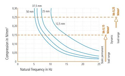
Natural frequency of a system consisting of a rigid mass and a layer of ISOLDYN® on a rigid base. Form factor q=3.
