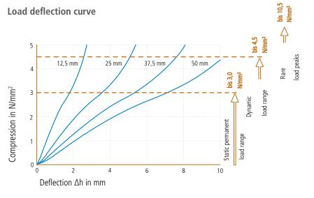
Spring characteristic curve. Test speed v = 1 % of thickness. Test at room temperature between flat steel plates. Recording of the 3rd load. Form factor q = 3.
