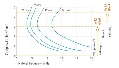
Natural frequency of a system consisting of a rigid mass and a layer of ISOLDYN® on a rigid base. Form factor q = 3.
