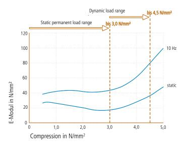
Load dependence of the static and dynamic moduli of elasticity. Dynamic E-modulus: harmonic excitation with an amplitude of  $\pm$  0.11 mm at 10 Hz and  $\pm$  0.04 mm at 30 Hz. Static E-modulus: tangent modulus from the spring characteristic. Measurement according to DIN 53513. Form factor q = 3.
