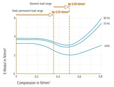
Load dependence of the static and dynamic moduli of elasticity. Dynamic E-modulus: harmonic excitation with an amplitude of  $\pm$  0.11 mm at 10 Hz and  $\pm$  0.04 mm at 30 Hz.
