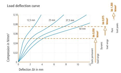
Spring characteristic curve. Test speed  $\nu=1$  % of thickness. Test at room temperature between flat steel plates. Recording of the 3rd load. Form factor q=3.
