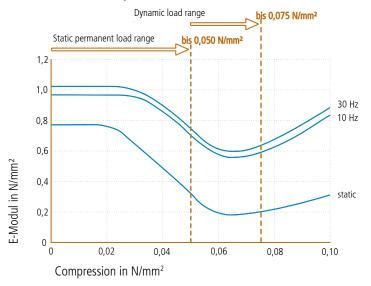
Load dependence of the static and dynamic moduli of elasticity.
