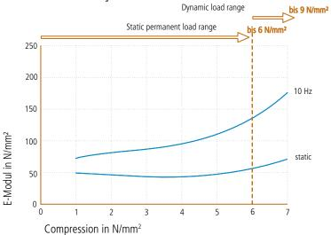
Load dependence of the static and dynamic moduli of elasticity. Dynamic E-modulus: harmonic excitation with an amplitude of  $\pm$  0.11 mm at 10 Hz and  $\pm$  0.04 mm at 30 Hz.
