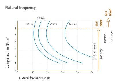
Natural frequency of a system consisting of a rigid mass and a layer of ISOLDYN® on a rigid base. Form factor q=3.
