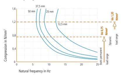
Natural frequency of a system consisting of a rigid mass and a layer of ISOLDYN® on a rigid base. Form factor q=3.
