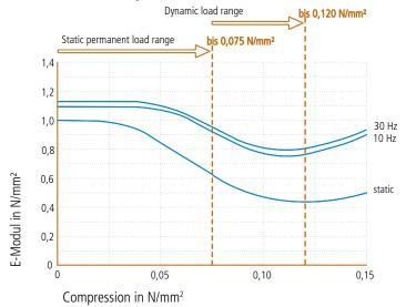
Load dependence of the static and dynamic moduli of elasticity. Dynamic E-modulus: harmonic excitation with an amplitude of  $\pm$  0.11 mm at 10 Hz and
